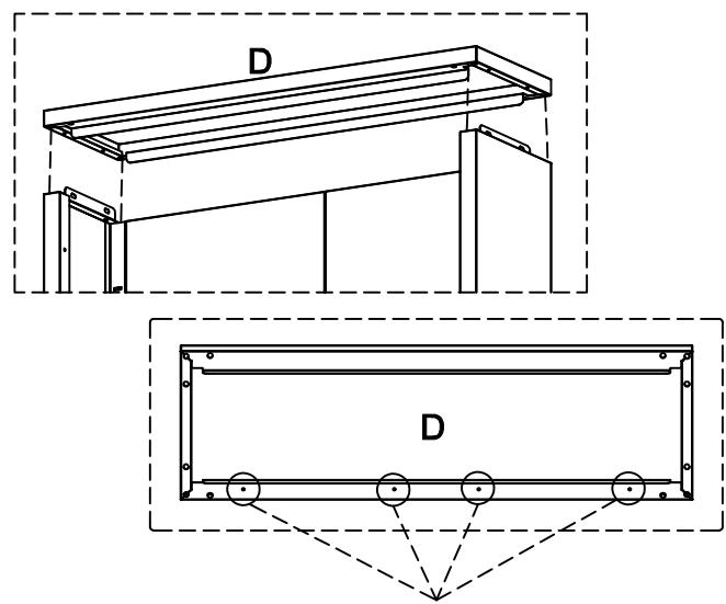
⚠ The back side of (D) with these 4 screw holes
